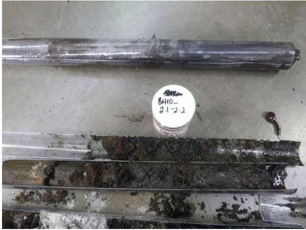
Example of mixed/variable filling material at borehole BH10.
