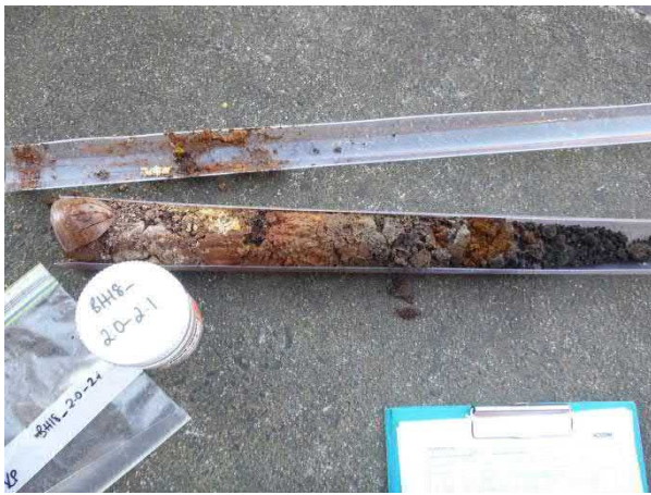
Example of mixed/variable filling material at borehole BH18.
